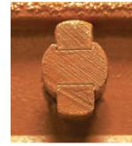
The 3-piece cross-rod assembly used in pultruded grating forms a strong, unified panel that can be cut and fabricated like a solid sheet. This unique system consists of two continuous, pultruded spacer bars and a center core wedge. The spacers are notched at each bearing bar so that the bars are both mechanically locked and chemically bonded
