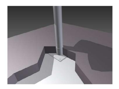
If there is no floor recess, you can start directly pushing the stairs. Please make sure that you start with stair 1. This stair has a shortened tube jointing sleeve that compensates the foot-plate thickness.
