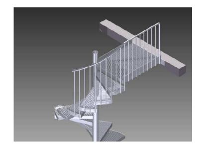
After all the railing segments of the staircase have been assembled, the assembly of the other landing railing can take place.
