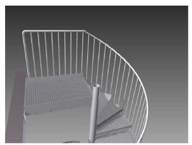
At the end of the finish post, a fixture for the platform railing is welded on. The platform railing can now be mounted between the wall and the post.
