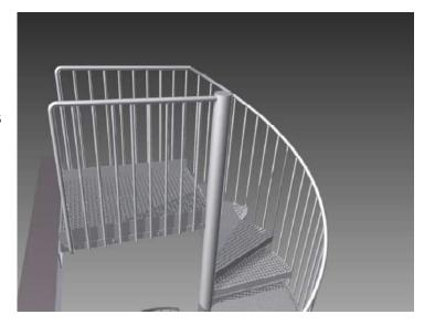
Start by sliding on the next standpipe element (Pos. 1/1...).
