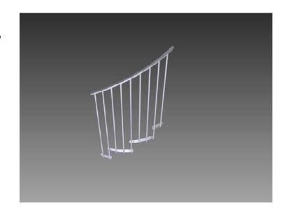
The handrail joints can be connected to the insertion inner tubes. The connecting flat bars at the handrail joint are made with half the length, so that they reflect a complete connecting flat bar when assembled.
