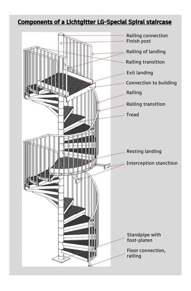
The LG- special type uses the "push-over sleeve" technique in its construction. Tube jointing sleeves are welded to the stairs and landings. They are pushed as a whole over the standpipe and then fixed in their predetermined position by mounting the railing.
