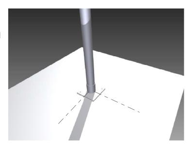
Set up the standpipe plumb. In case of multi-part standpipes, the lowest standpipe is always marked with pos. 1. If a floor recess is planned, we supply a loose tube jointing sleeve as a spacer tube (pos. 6), which compensates for the floor recess.
