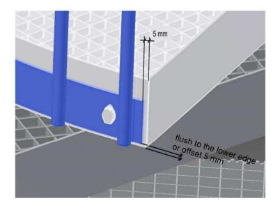
Staircase diameter 1200 – 1700 mm = flush to the lower edge Staircase diameter 1800 – 3300 mm = 5 mm Observing these features, all railing segments must be installed from top to bottom.
