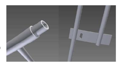
The railing segments have an item number stamped on the connecting flat bars. The first segment with the "marking 1" must be assembled together with the second railing segment "marking 1" (1 to 1; 2 to 2; ...).
